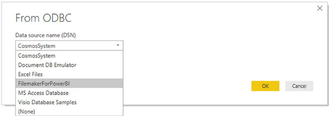
Figure 6-20. The Power BI Desktop From ODBC dialog to select an ODBC data source
